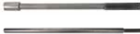
Devices for checking barrel straightness and elongation of the cartridge chamber (various calibers)
